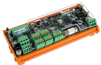
In specific applications more than one position transducer may be required. Four additional potentiometric transducers inputs are available on the module for that purpose.
