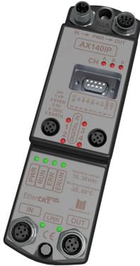
AX140IP is an slave module EtherCAT with an isolated input to read incremental encoder; the encoder is supplied directly from the module. Four digital inputs are available to read proximity, switches, push-button etc.
